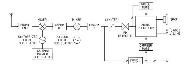
Figure 2.1 T855 High Level Block Diagram
