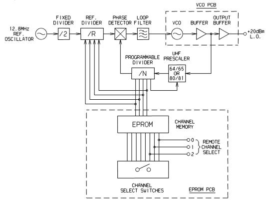
Figure 2.5 T855 Synthesiser Block Diagram
