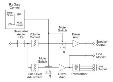
Figure 2.3 T855 Audio Processor Block Diagram
