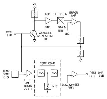
Figure 2.6 T855 RSSI Block Diagram
